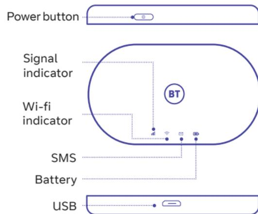
**Note:** The battery LED will light up when the device is powered on.
