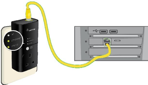
Shortly, you will see the Ethernet LED blinking; this indicates that there is data traffic going through the PG9020. You are now ready to start using your network.
