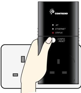
**Step 2:** Reset the new Adapter to its factory settings: this is to make sure your new adapter is set as an EP (end point). Press the CONFIG/RESET button for 10 seconds. All LEDs will turn OFF and the STATUS LED will be RED.
