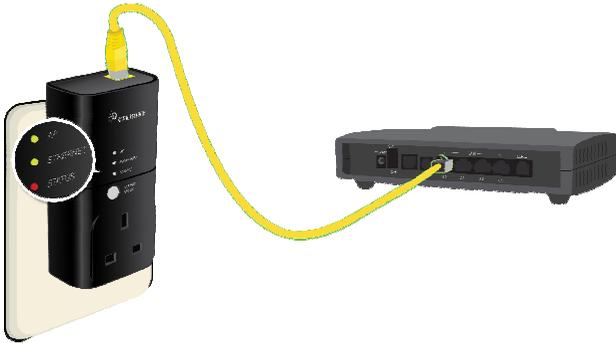
Connect the other PG9020 to your Computer, Game Console, Set Top Box or other network device using an Ethernet cable. This is the End Point (EP).
