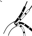
First remove the cable clamp. Connect the 2 exposed wires into the first set of twin screw connectors in your Ultimate 106 and tighten the screws to secure the wire, in place.
