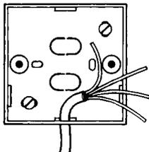
Run the required cable length to your Ultimate 106. Attach the cable firmly to the wall.
