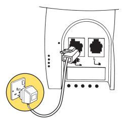
Plug the power adaptor into the mains power socket and switch on. The green Power/In Use light comes on.
