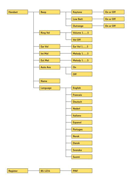
Important. If you make a mistake you can return to the previous menu heading by pressing the ★ button. If you press and hold the ★ button at any time you will return to the standby screen. After 30 seconds if no buttons are pressed the handset will automatically return to the standby screen.
