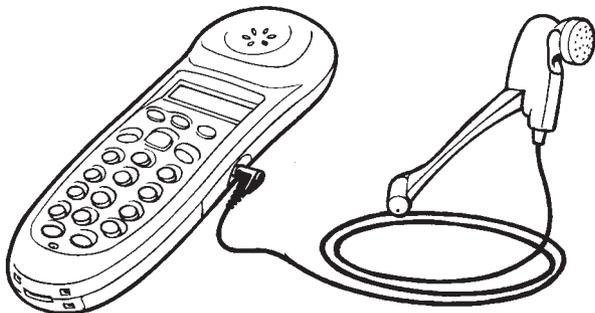
Remove the small cover and plug the headset into the socket on the side of your Synergy 1000.
