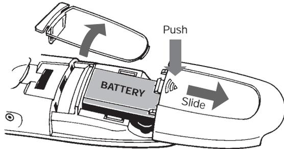
Insert the battery pack inside the battery compartment and slide the battery compartment cover shut. Replace the directory label cover.
