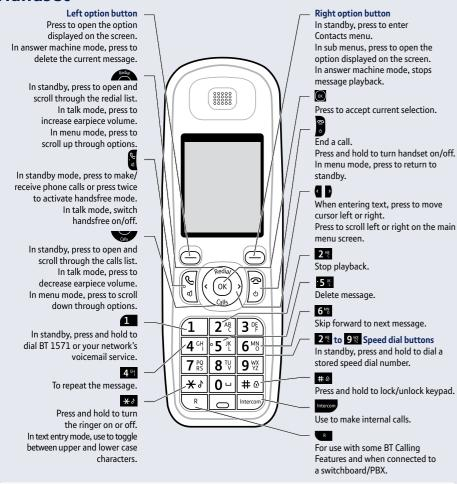
The answer machine handset controls on buttons 24 44 55 and 65 will only work when a message is being played on the handset.
