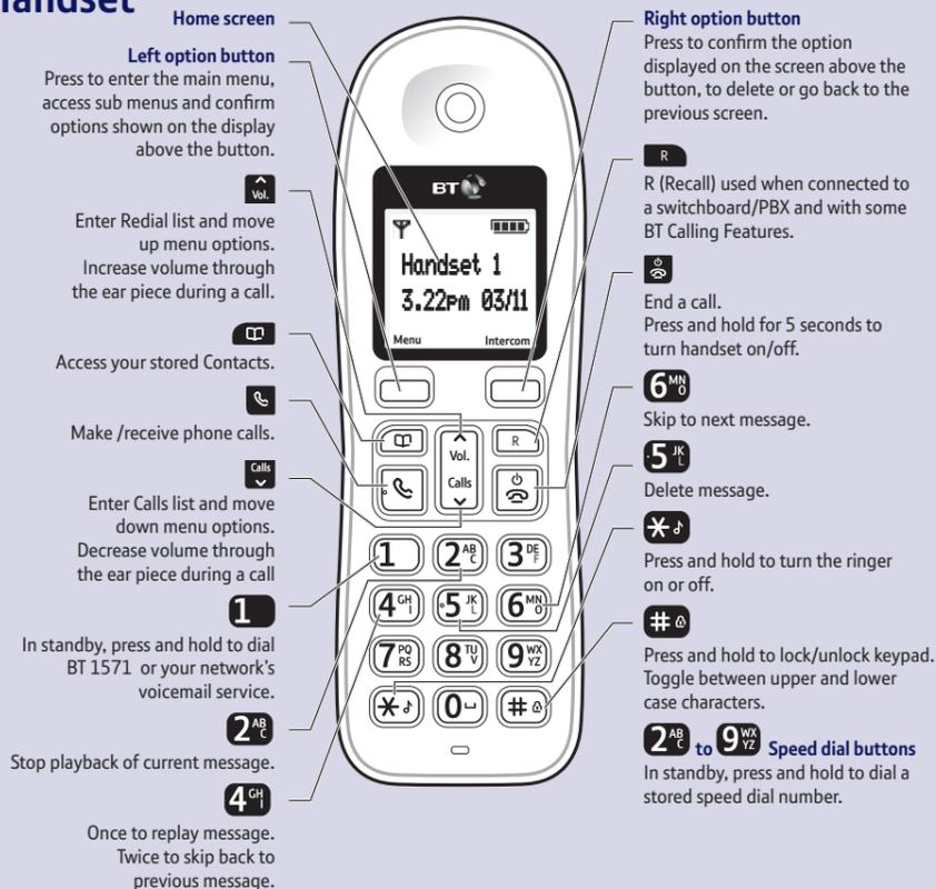
The answer machine handset controls on buttons **2<sup>AB</sup>**, **4<sup>GH</sup>**, **5<sup>JK</sup>** and **6<sup>MNO</sup>** will only work when a message is being played on the handset.
