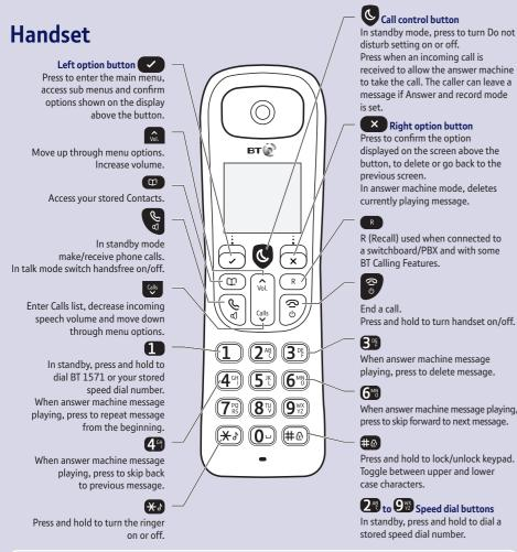
The answer machine handset controls on buttons **1 4 3** and **6** will only work when a message is being played on the handset.
