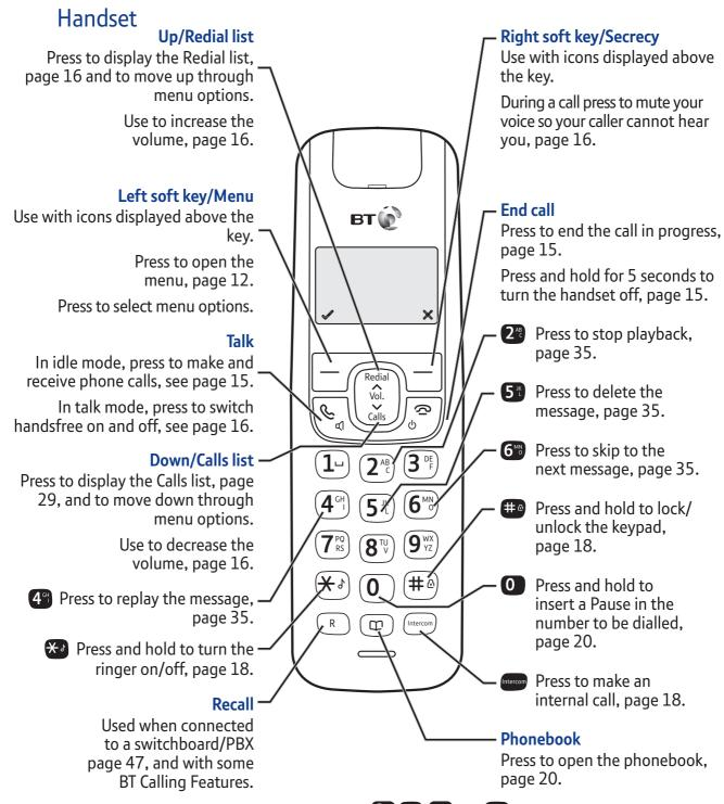
The answer machine handset controls on buttons 2° 4° 5° and 6° will only work when a message is being played on the handset, page 35.
