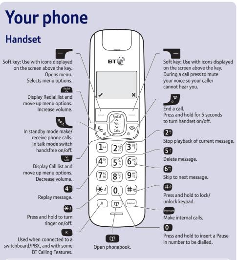
The answer machine handset controls on buttons 2 4 5 and 6 will only work when a message is being played on the handset.
