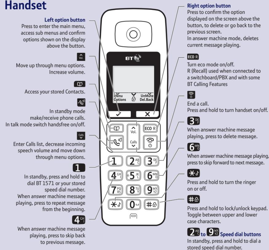
The answer machine handset controls on buttons **1**, **4**, **3** and **6** will only work when a message is being played on the handset.
