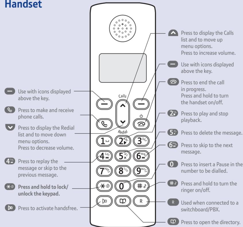
The answer machine handset controls on buttons **2**, **4**, **5** and **6** will only work when a message is being played on the handset.
