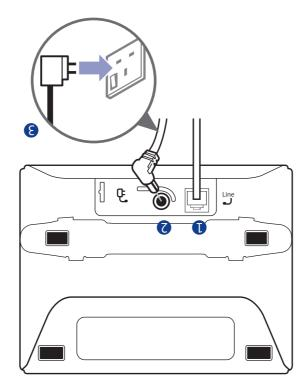
wall socket and switch on. power adaptor into the 3 Plug the other end of the
