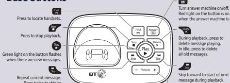
Press twice to skip to previous message. In use charging light Blue light is on and flashes when phone rings or the handset is in use
