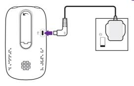
mains power socket and switch the socket on. 1 Plug the cable into the Parent unit, then plug it into the
