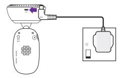
mains power socket and switch the socket on. 🚯 Plug the cable into the Baby unit, then plug it into the
