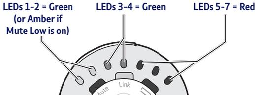
The seven LEDs across the top of the Parent unit light up to indicate the level of sound being received from the Baby unit. The LEDs light up progressively as the sound increases.
