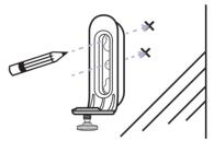
2. Remove the wall mounting bracket and check the reception strength of the Baby unit and camera angle before drilling two holes in the wall using a 5mm drill bit.
