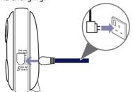
4. Leave the battery to charge continuously for 12 hours before you switch the Parent unit on. When the battery is fully charged the light on the side of the Parent unit will turn off.
