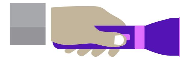
This is similar to how data is sent through an optical fibre... in this activity the torch was the transmitter, but in digital communications your Wi-Fi router sends light pulses down the optical fibre instead. When the data is received at the other end, it is decoded into binary 1s and 0s which the computer understands and can display on-screen – just like you ‘decoded’ the animal names.
