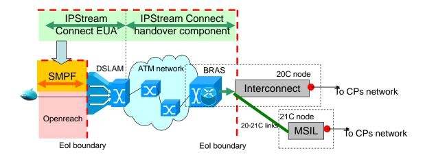
BT IPStream Connect End user Access products: BT IPStream Connect Handover Component, with option of interconnect at 20C node or 21C node (via MSIL)
