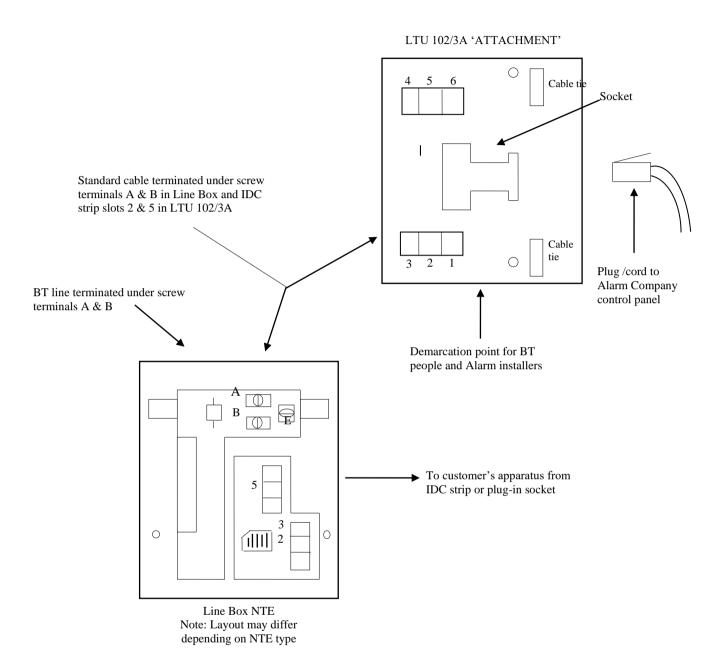
Figure 2 An Explanatory Picture of an Interface using LTU 102/3A
