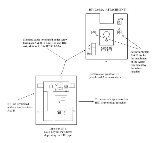
Figure 1 An Explanatory Picture of Interface using BT 80A/92A.
